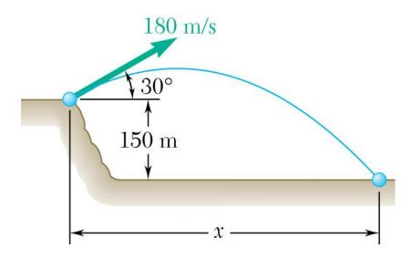
A projectile is fired from the edge of a cliff with an initial velocity of 180m/s with 30° angle with the horizontal. Neglecting air resistance, find:
