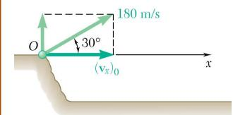
For the horizontal motion substitute the initial velocity into the uniform motion equation.
