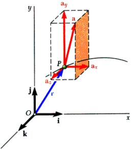
• When position vector of particle *P* is given by its rectangular components,
