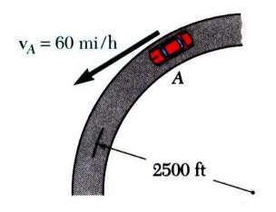
A motorist is traveling on curved section of highway at 60 mph. The motorist applies brakes causing a constant deceleration rate.
