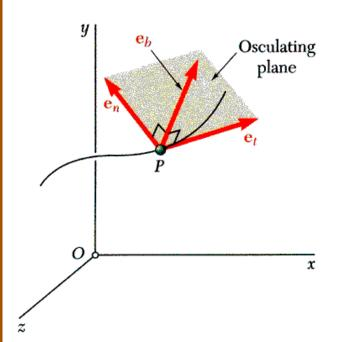
• Relations for tangential and normal acceleration also apply for particle moving along space curve.
