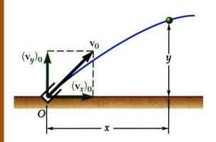
• Rectangular components particularly effective when component accelerations can be integrated independently, e.g., motion of a projectile,
