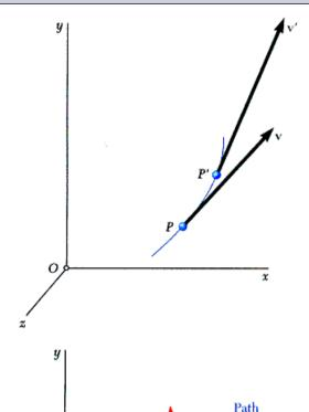
• Consider velocity  $\vec{v}$  of particle at time t and velocity  $\vec{v}'$  at  $t + \Delta t$ ,
